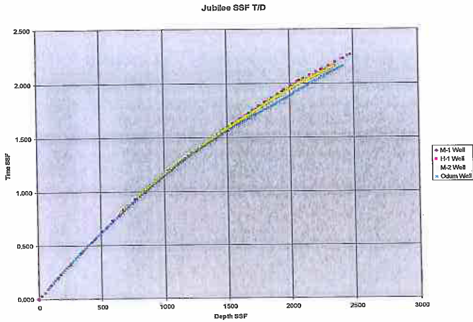
Figure 32: Time-Depth Curve (below mudline) for Jubilee Field Wells
